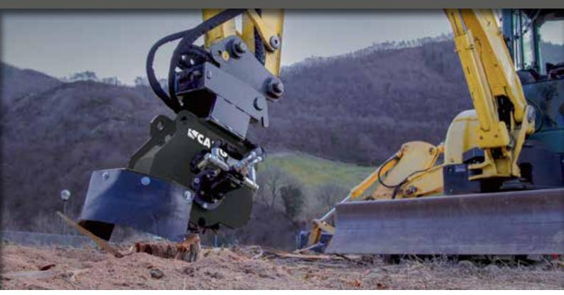
FAST AND EFFECTIVE, THIS ATTACHMENT GRINDS STUMPS AND WOOD EVEN IN DEPTH; THE SHREDDING WHEEL SWINGS FROM SIDE TO SIDE AND GRADUALLY EATS INTO THE STUMP UNTIL IT HAS BEEN COMPLETELY ELIMINATED. THE DIRECT DRIVE WITH PISTON MOTOR DELI-VERS THE HIGHEST CUTTING SPEED AND THUS OPTIMAL PRODUCTIVITY AND EFFICIENCY. THE TUNGSTEN CARBIDE TEETH ARE EXTREMELY TOUGH.
