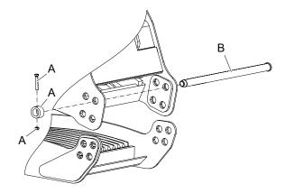
Remove the adjusting pin (B).
