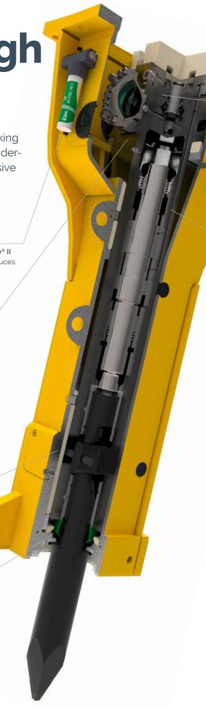
The built-in pressure cut-off valve **PowerAdapt** prevents overloading.
