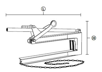
Designed to improve safety when transporting or laying pipes. The strong profiled beam will fit all pipes up to 3000mm length.
